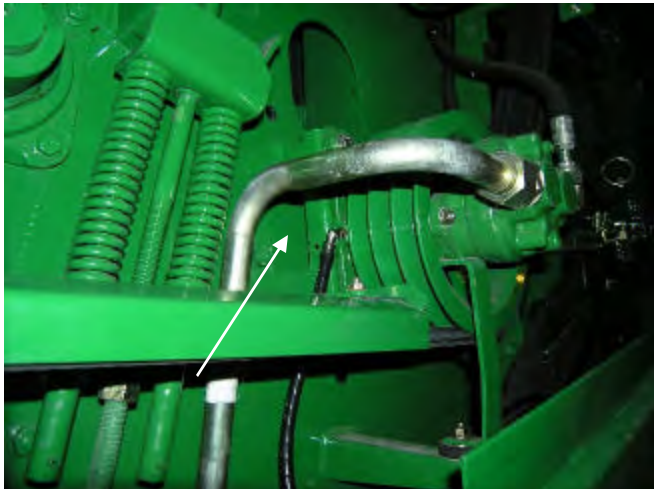
Install one 244054 fitting into Reel Drive Pump port. Route/install tubing from outlet 7.
