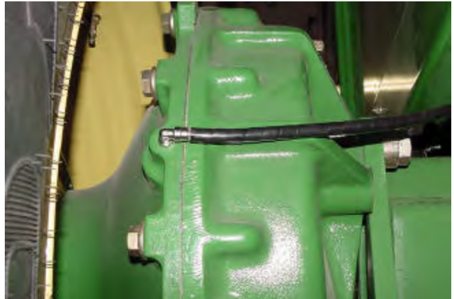
Install one 243699 fitting in Final Drive Outer Bearing port. Route/install tubing from outlet 1.
