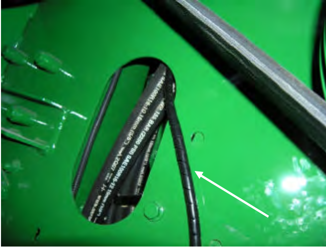
Route feed line for Discharge Beater Bearing through oval cut-out and follow hydraulic hoses to top of machine.
