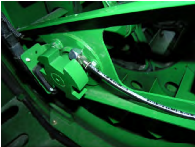
Close-up of line routing. Keep line tight to frame.
