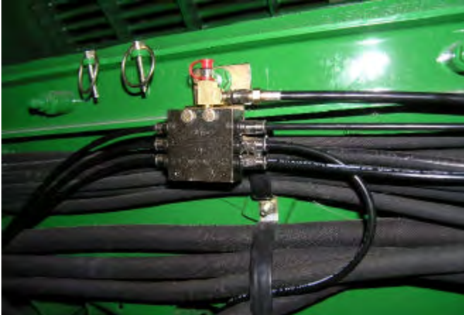
Mount Left Front Secondary Valve below separator covers as shown in picture above. Use existing hardware for mounting valve bracket.
