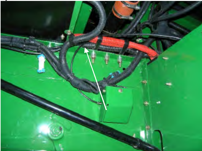
Split lines above the Discharge Beater Bearing. Install #244053 fitting in Discharge Beater Bearing port. Install tubing.
