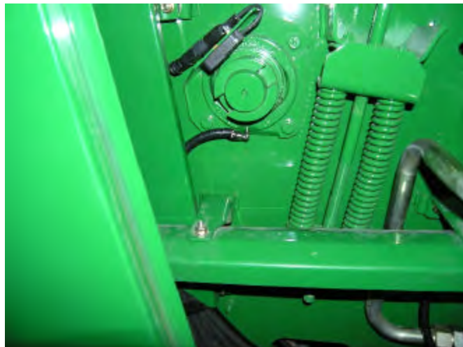
Install one 244053 fitting in Feed Accelerator Bearing port. Route/install tubing from outlet 6.
