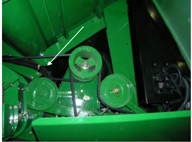
Combine supply line and Discharge Beater Bearing lines at top of machine behind belt pulleys. Route lines along existing hydraulic lines.
