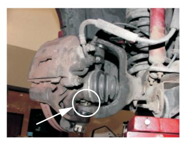
Lincoln's Model 5883 Special Access Coupler provides an efficient way to lubricate fittings in tight locations
