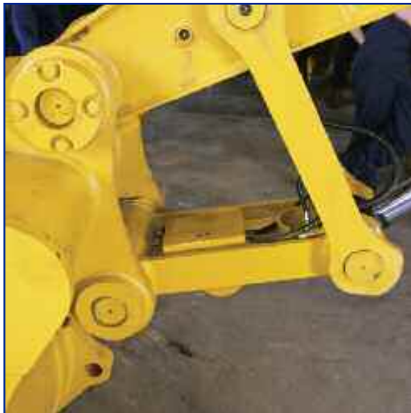
VALVE #3 Serving: H-link and bucket linkage. The valve guard has been added to the H-link.
