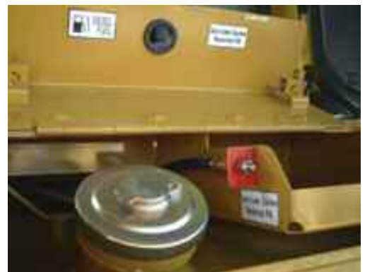
Ground level reservoir filling is made easy with optional remote fill fitting
