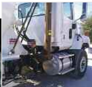
Quicklub system installed on a ready mix truck
