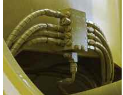
Quickclub® metering valves ensure more grease is delivered to high-demand bearings
