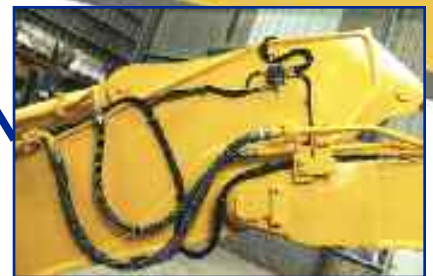
VALVE #2 Serving: Bucket cylinder foot pin, arm link pin, arm cylinder (rod end), boom arm pin and arm bucket pin
