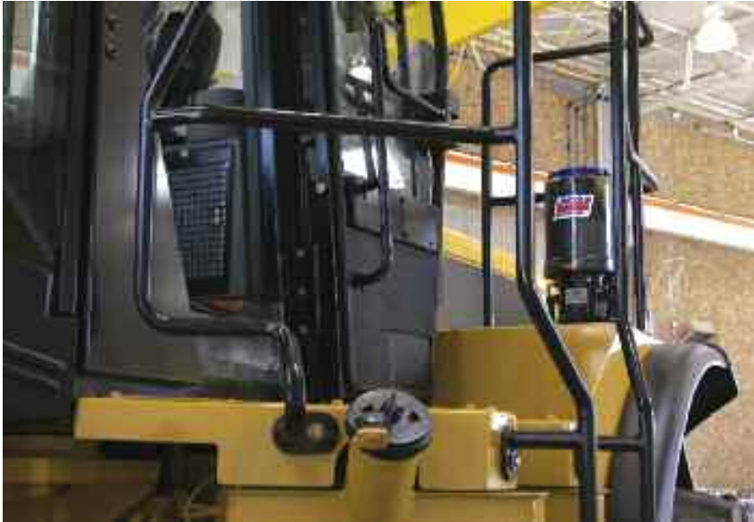
On this loader, a Quickclub pump is mounted on the operator deck/fender near the cab for ease of visual monitoring and service
