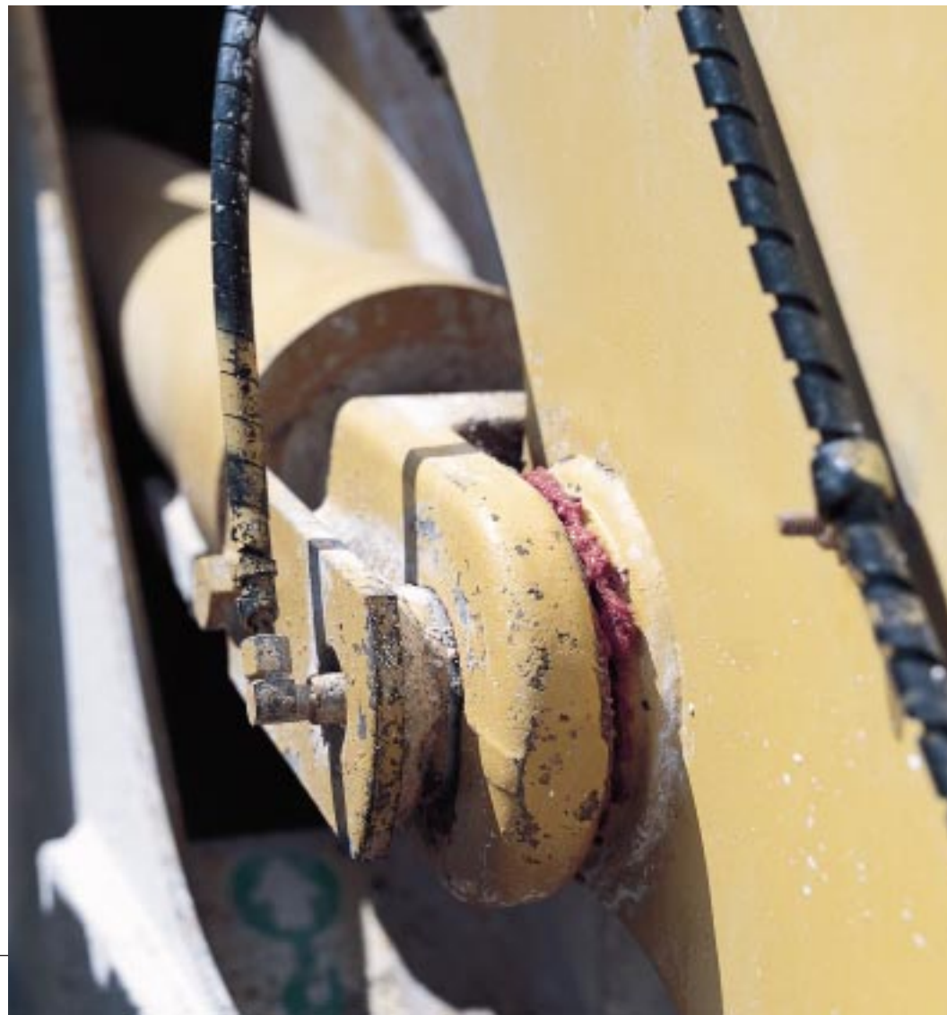
Lift arm with grease seal
