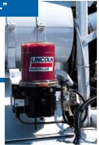
The pump works with standard NLGI grease No 2.
