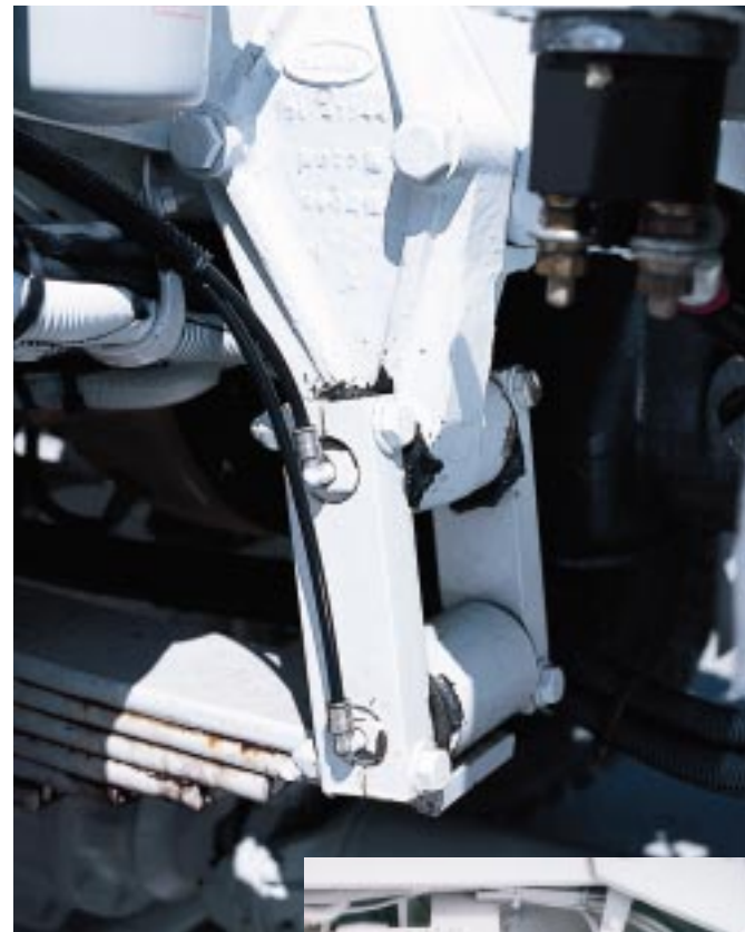
Quicklinc fittings are the only press-to-lock ones on the market with high pressure capability.
