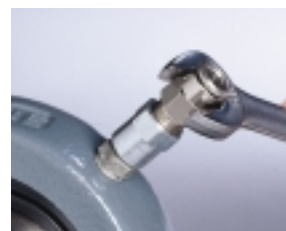
4. Then thread a Quickline completely into the Zerk-Lock
