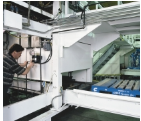
Total installation and start-up time for this 10-lubrication point palletizer using NLGI #2 grease was only four hours. The satisfied customer ordered two QLS 301 systems long before the product's release.
