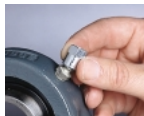
2. Place a Zerk-Lock onto the fitting
