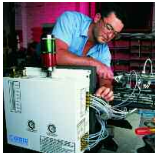
Greg Hoag, a field erector for Marshall and Williams Company, prepares an ORSCO 150 unit for installation in the conveyor system of a textile mill in Mexico City.
