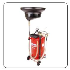
Model 3635 gravity drain has a portable upright configuration commonly used for collecting fluids under lift-mounted vehicles. It offers a 15 in. (381 mm) offset funnel that includes a removable filter screen and wide-mouth extension that increases the diameter to 24 in. (610 mm). Height is adjustable from 51 to 76 in. (1,3 to 1,9 m), not including the extension.
