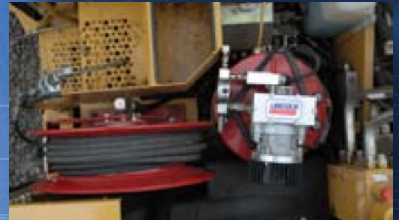
TOP VIEW OF REEL-N-FLOW INSTALLATION
