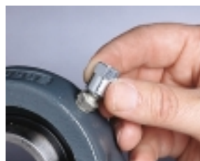
2. Place a Zerk-Lock onto the fitting
