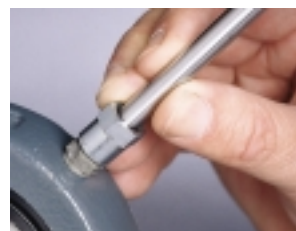
3. Seal and tighten Zerk-Lock using a hammer and staking tool
