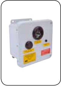
Control box with grease-level gauge (24 V DC), "full" light and momentary switch for shut-off valve.
