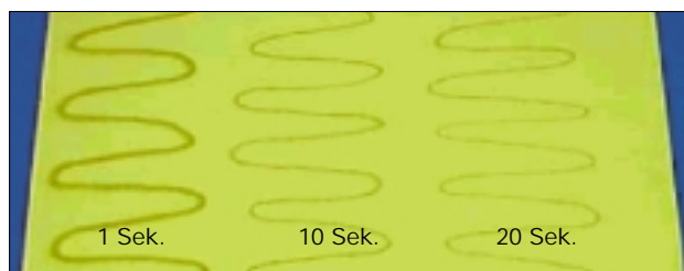
The spray patterns beside show 1/2 drop of lubricant dispensed over 1 second, 10 seconds and 20 seconds.
