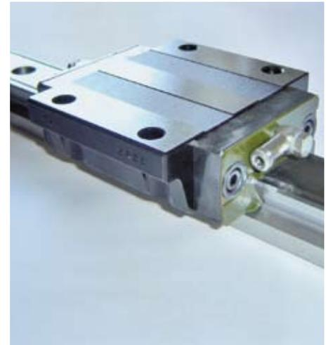
**A large portion of industrial movements are linear. This includes, for example, the transportation of components within an area, or the feeding of tools to the work-piece – or vice versa. Such guiding systems must be supplied regularly and evenly with an optimal amount of lubricant. Usually the manufacturers of linear guides will indicate in their data sheets at what interval lubricant should be supplied to the linear guide carrier.**
