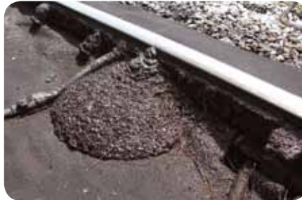
Competitor's wiper bar – clogged ports divert grease to the ONLY open lube port
