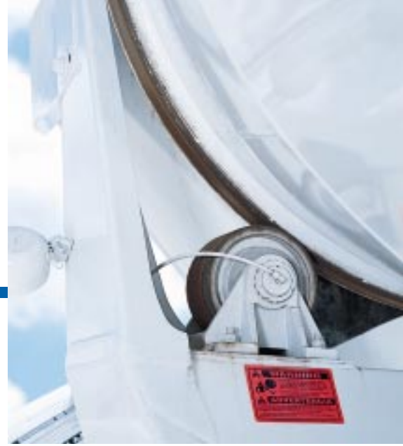
Drum roller failures caused the highest maintenance costs before automated lubrication.
