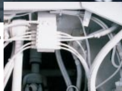
One-piece SSV divider valves have no weak points compared to other segmented metering valves.
