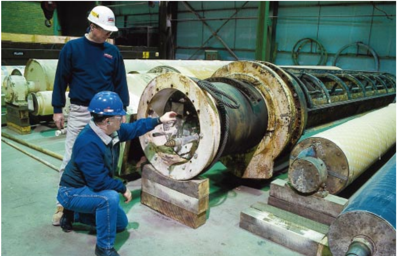
RAY DOLAN AND DOUG BELL LOOK OVER THE #2 COUCH ROLL BEARING AFTER INSPECTION.
