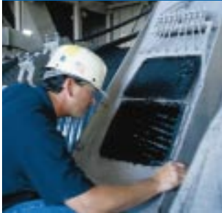
Don Fithian, Lincoln Industrial National Accounts Manager, Construction and Mining, looks into the open gear lubrication on a Bucyrus 1570 dragline's hoist rope.
