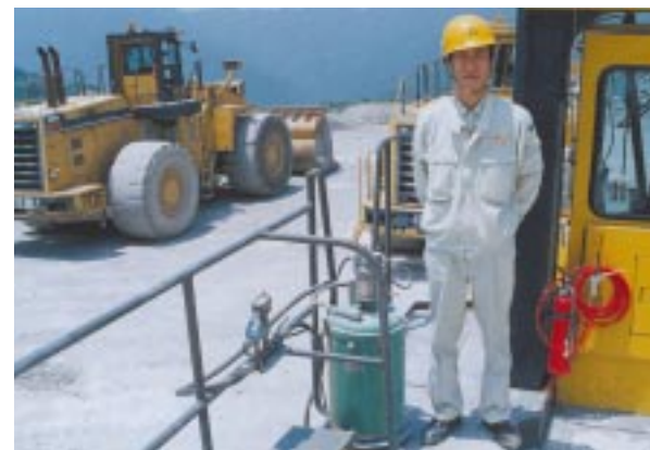
992G Cat loader uses Centro-Matic® grease system with a hydraulically operated pump.
