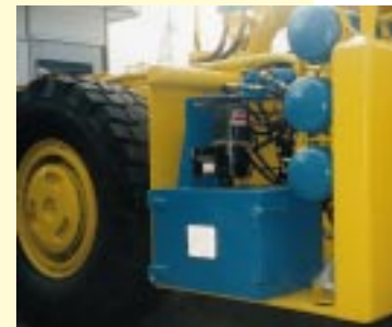
Quickclub® pump system on a Boart-Lena SWWN 7H drilling machine.
