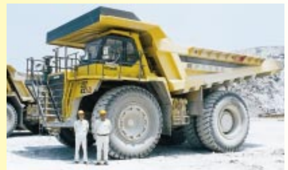
Masaaki Shibata (left) and Tahito Koyama oversee Todaka's mining vehicles. Todaka's Komatsu HD785 and HD985 dump trucks increased their working time a half-hour each week with Centro-Matic®.
