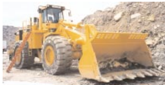
992G Cat loader uses Centro-Matic® grease system with a hydraulically operated pump.
