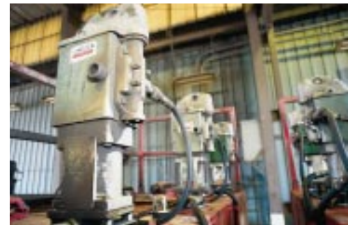
Seven PowerMaster® pumps are on each Kindill lube truck. Some also have a lower ratio pump tube for transferring oil.
