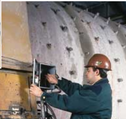
QLS 301 being programmed from machine's existing PLC.
