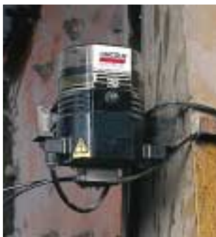
QLS 301 being programmed from machine's existing PLC.
