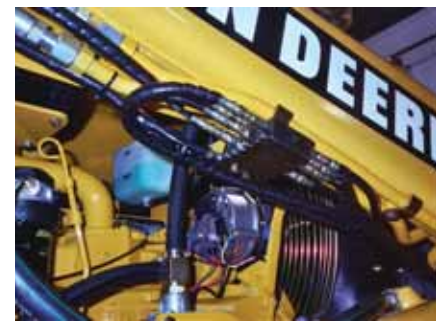
Line routing and protection are critical to reliability.
