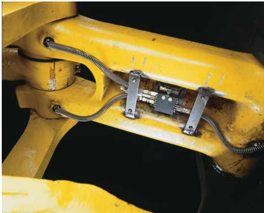
A constant supply of grease and lubricant when the machine is moving means contaminants are kept out and all wear surfaces are protected.
