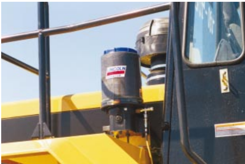
This Caterpillar 980G wheel loader is equipped with a lubrication system powered by a Lincoln Quicklub 203 pump with 8-liter reservoir.
