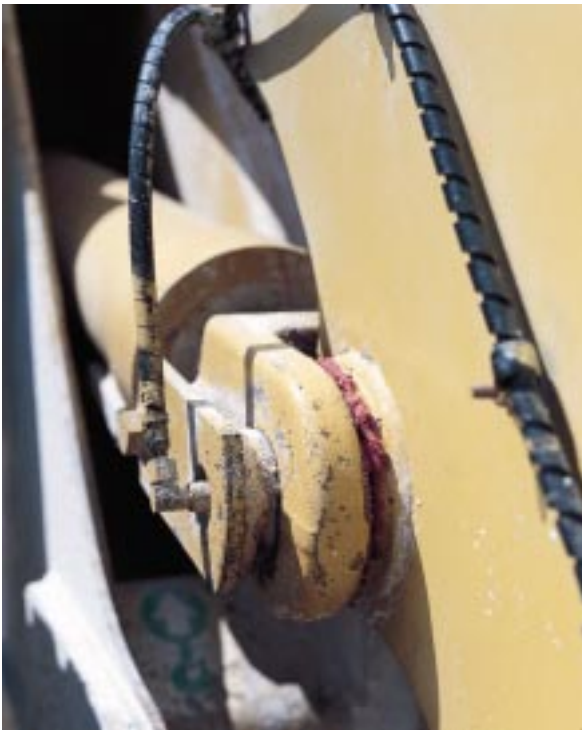
A perfect grease seal is visible on this wheel loader lift arm.
