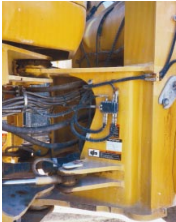
On this machine, the primary valve is mounted on the right-hand front frame. A 1/8-in. high-pressure hose is protected by spiral-wrapped guarding and spring coils.
